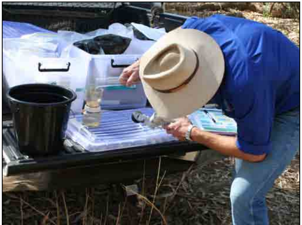
DON'T MESS WITH MY PROCESSES: South West NRM's GIS and Property Officer, Daniel Wingett uses a Nalgene filtering kit at one of the testing sites for chlorophyll A analysis of the water sample.
