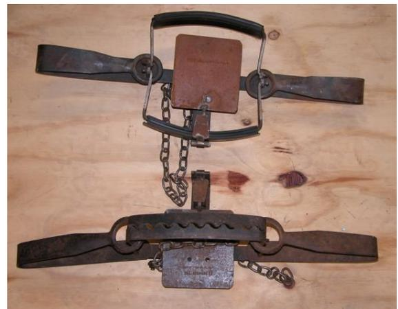
**Lane's traps padded (top) and standard with teeth (bottom). Lane's traps have a 21 cm jaw spread.**
