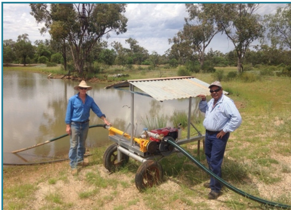
Above: Col Creagh of Varna and Kevin Collins of South West NRM inspect a mobile transfer pump used to pump water to off-stream troughs to reduce grazing pressure in the Paroo river Catchment.
